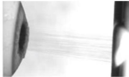
**Speed of delivery:** Our piezo-print technology is similar to high-precision ink-jet printing. Unlike a simple aerosolized mechanism, the Optejet is designed with ejection control that creates a fast and targeted micro-jet delivery. Solution is dispensed to the ocular surface in less than 100 milliseconds between the time the first droplet hits the corneal surface to the completion of dose delivery, which is faster than the average involuntary blink response time.
